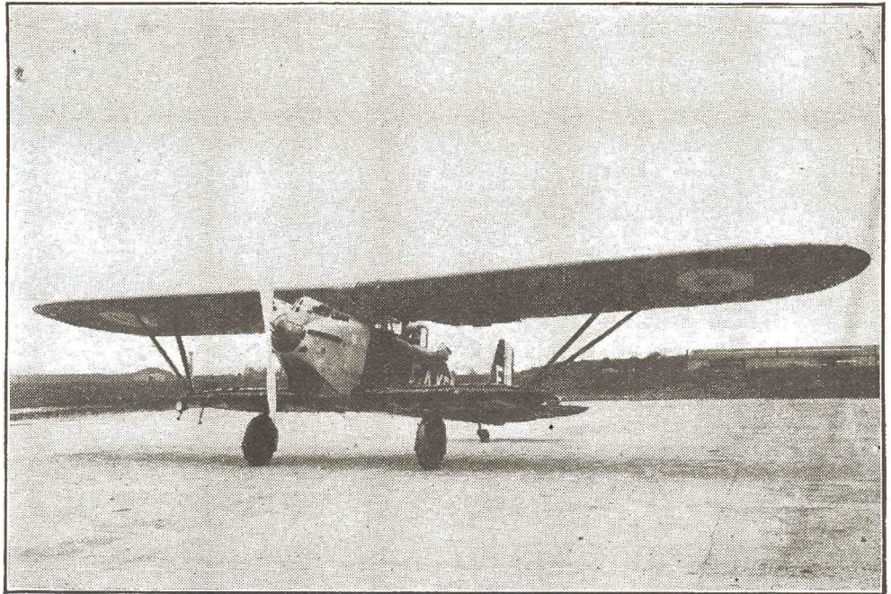
The modern Spad, now listed in the Jockey interceptor class. This high-speed single-seater is made by the Bleriot Company of France and is now regular equipment in the French Air Service. With a 500 C. V. Hisso, it carries two Vickers guns and does well over 200 m.p.h. The type number is S-91-C.8.
