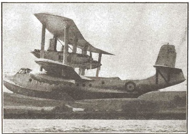
The latest addition to the R.A.F. flying boat squadrons—and already in use in the colonies. This is the Short "Singapore" Mark 111 ship completed last year. It is powered with four special Rolls-Royce motors suitably geared for tandem settings. It can fly on two engines, and carries two pilots and two gunners.
