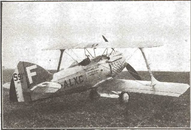
The modern Spad, now listed in the Jockey interceptor class. This high-speed single-seater is made by the Bleriot Company of France and is now regular equipment in the French Air Service. With a 500 C. V. Hisso, it carries two Vickers guns and does well over 200 m.p.h. The type number is S-91-C.8.
